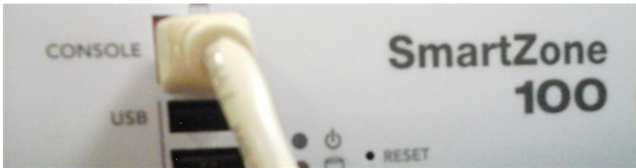
Figure 1. Location of console port
